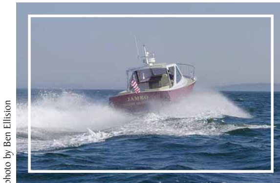
Jambo , hull #002, with twin jet-propelled 300-hp. Yanmars
